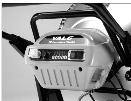
Unscrew two screws and take the burner cover off
